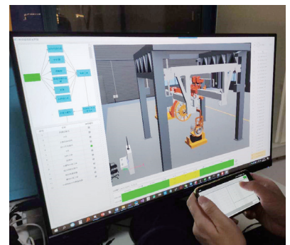
图12 单模块装配工艺过程人在回路仿真 Fig.12 Process simulation with man-in-loop of typical assembly module
